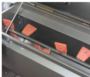
Destemmer shaft with rubber tips
